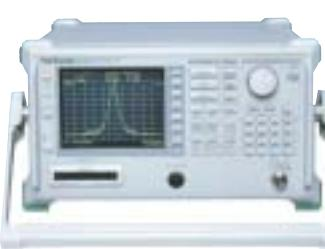
This portable spectrum analyzer allows measurement of spurious frequencies of up to three times greater than the frequency bands used worldwide for mobile communications.
