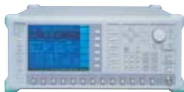
A high-performance digital modulation signal generator that incorporates a broadband vector modulator.
