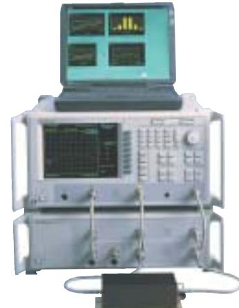
With power handling capabilities up to 100 Watts, this turn-key system dramatically simplifies the test complexity of both base station and handset power amplifiers between 800 and 2400 MHz.
