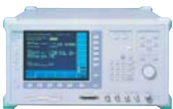
Supports the test needs of the manufacturing, R&D, and maintenance markets in multiformat testing including IS-95, GSM, DCS 1800/PCS 1900, IS-136A, AMPS/NAMPS, PDC, and PHS.
