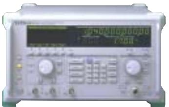
With high signal purity, these signal generators are ideal for radio receivers interference testing, as sources for various local and reference signals.
